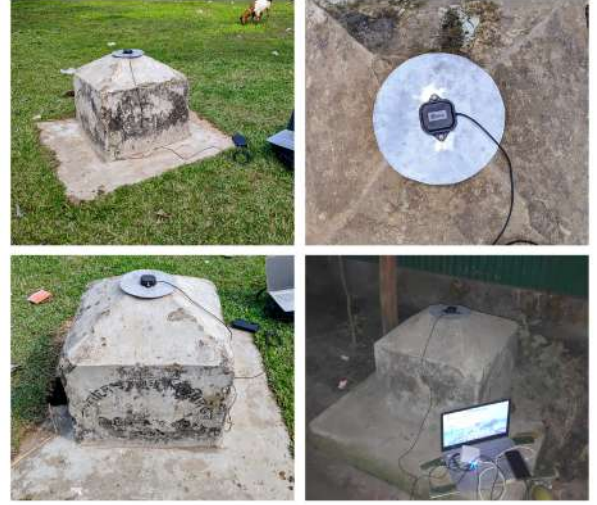
Fig. 3. U-blox ANN-MB GNSS antenna mounted on a 15cm circular ground plane and placed on top of the geodetic control point which is connected to the GNSS survey grade receiver (Ardusimple simpleRTK2B Budget).
