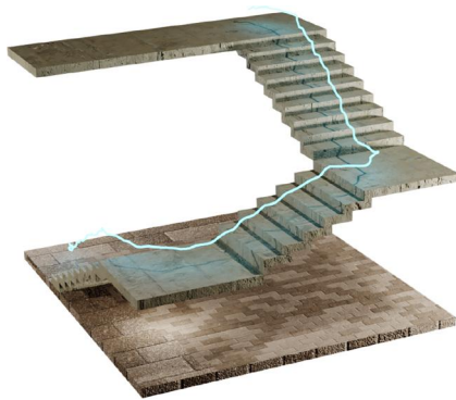
FIG. 26. Experimental results: Climbing stairs with monocular visual-inertial state estimator. Trajectory overlaid over stairs for visual comparison.
